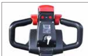
Multi-function handle with butterfly switches & LCD display
