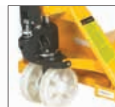
Sealed hydraulic pump unit
