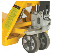
Sealed hydraulic pump unit with nylon tyred steering wheels
