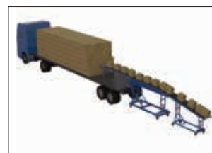
High rise telescopic conveyor with adjustable extension
