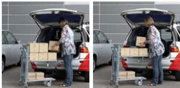
Spring loaded shelf maintains a constant height when loading/unloading
